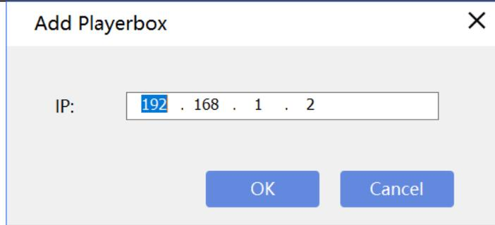
Figure 4.4-10 Manually adding terminals
