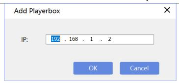
Figure 4.4-10Manually adding terminals
