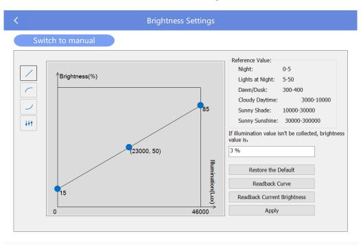
Figure 4.4-25Automatic brightness adjustment
