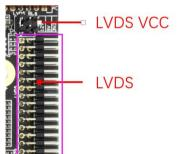
General LVDS interface definition, support single / dual, 6/8 / 10-bit 1080P LVDS screen. The screen voltage can be selected through a jumper cap, and it can be selected to support 3.3V / 5V / 12V screen power supply. In order to avoid burning boards and screens, please note the following: Please confirm whether the screen specification book screen supply voltage is correct, whether the board's corresponding power supply can meet the maximum working current of the screen.
