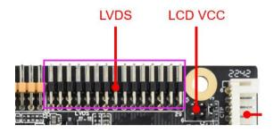
General LVDS interface definition, support single / dual, 6/8 / 10-bit 1080P LVDS screen. The screen voltage can be selected through a jumper cap, and it can be selected to support 3.3V / 5V / 12V screen power supply. In order to avoid burning boards and screens, please note the following:
