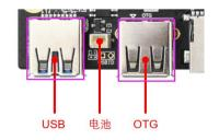
The board has 2 USB standard interfaces and 4 USB pins, one of which is shared with the 4G module.
