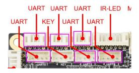
The board have to two sets of ordinary UART serial ports, which can support the UART serial port devices on the market.
