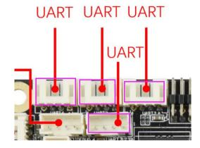
The motherboard leads to two sets of common UART serial ports, which can support common UART serial devices on the market.
