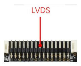
General LVDS interface definition, support single/dual, 6/8/10 bit 1080P LVDS screen. The screen voltage can be selected through the bridle-wire cap, and can choose to support 3.3V/5V/12V screen power supply.
