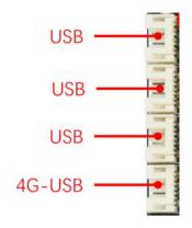
The motherboard has 2 USB standard interfaces and 4 USB pins
