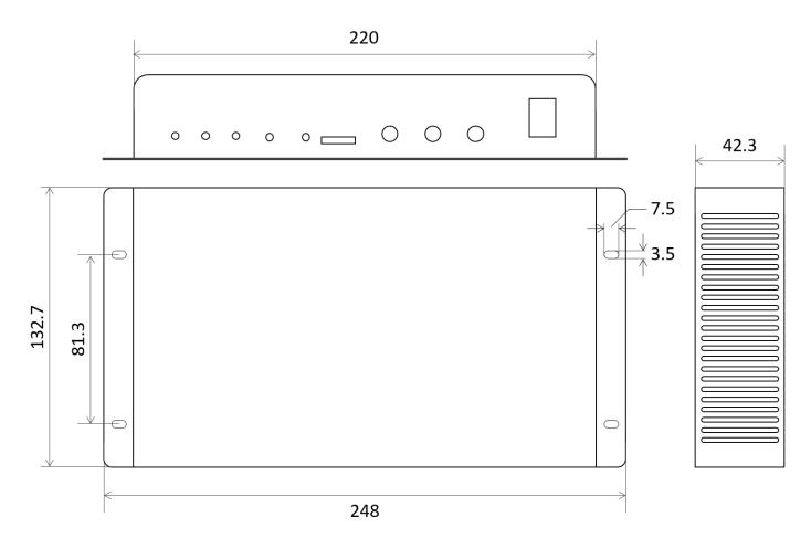
Tolerance: ±0.3 Unit: mm
