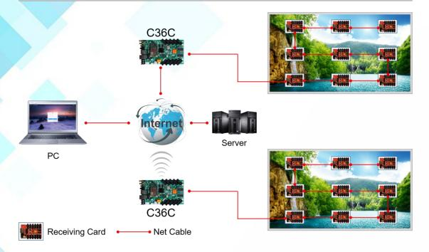
2. Asynchronous one-to-one control: Update programs by network cable connections, Wi-Fi connections or USB flash drives. LAN (cluster) control can access to the LAN network through network cable connection or Wi-Fi Bridge.
