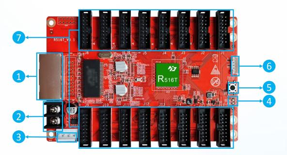
(1): Gigabit Ethernet port, used to connect the sending card or receiving card, the same two network ports are interchangeable,
