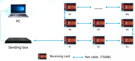
Connection diagram of connecting R516T with player A6:
