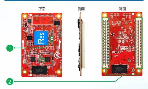
① Indicator light: RUN light is working light, the light flashes when the control card is working normally. D2 light is network light, net cable connects well and receiving card working normally, the light fast flashing.
