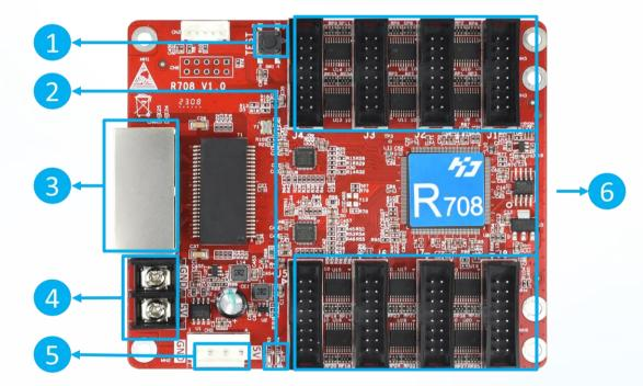
(1): Test button, used to test display brightness uniformity and display module flatness.
