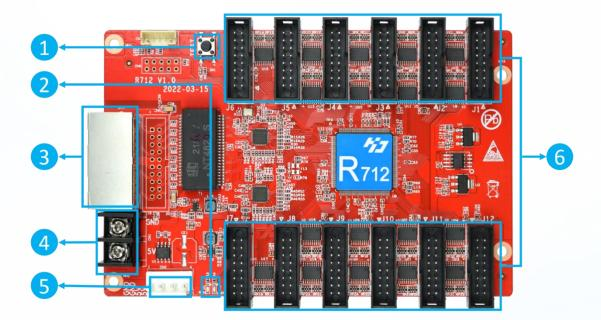
(1): Test button, used to test display brightness uniformity and display module flatness.
