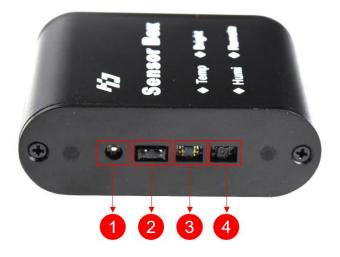
(1) **Running light:** flicker—work; not bright—Not working, Press the remote control and it will flash.
