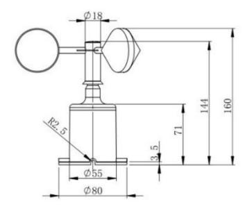
Overall height: 160 Spindle height: 144 Spindle height: 71 Base diameter: \$\phi80\$
