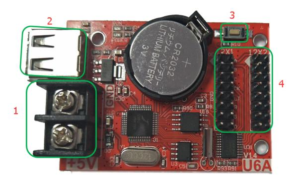
①: Power connector, connect 5V power supply;
