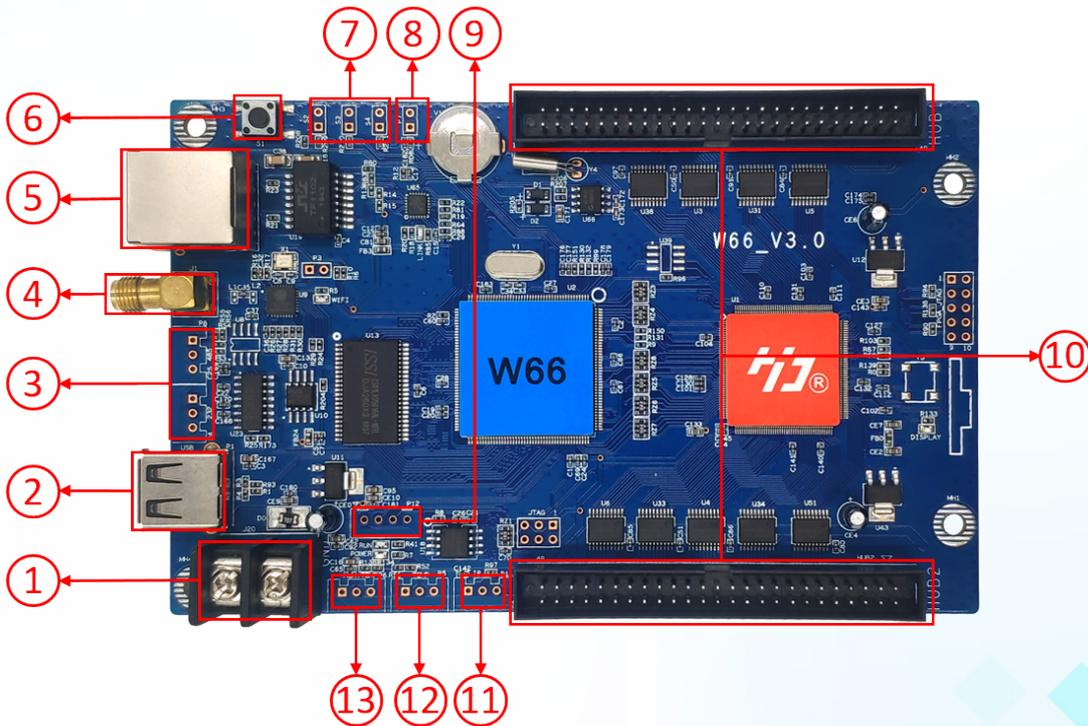
1. Power connector, connect 5V power supply
