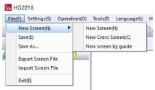
New screen (Ctrl+N): used to create a new screen(No screen counts limited), Can also be grouping manage(select group option in system setting).
