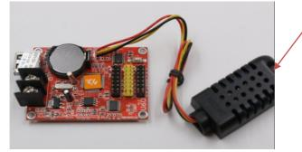
The Temperature+ Humidity parameter Type: AM2301 Working voltage: 4.2-5.2V Testing humidity range: 0-100%RH Testing temperature range:  $-40-80^{\circ}$ C Testing humidity precision:  $\pm 3\%$ RH Testing temperature precision:  $\pm 0.5^{\circ}$ C
