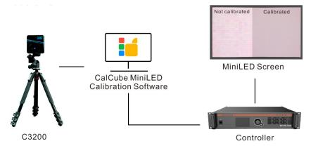
Main use: Pixel-level high-accuracy brightness and chroma measurement and calibration of MiniLED screens, microLED screens, etc.
