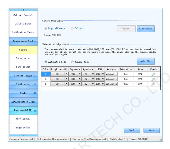
Fig. 4-8 Adjusting saturation of digital camera
