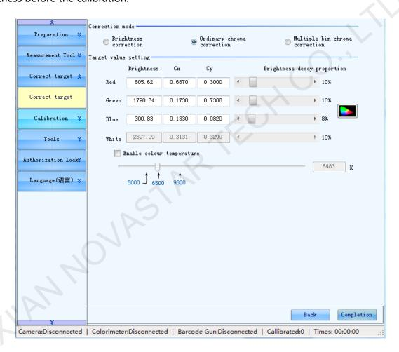
Fig. 4-12 Setting calibration mode and target value
