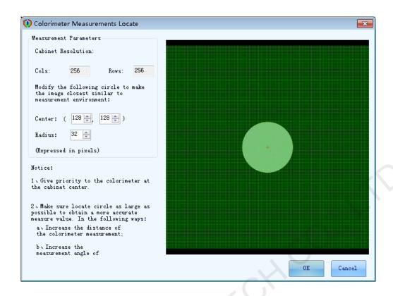
Fig. 4-15 Setting of measuring area
