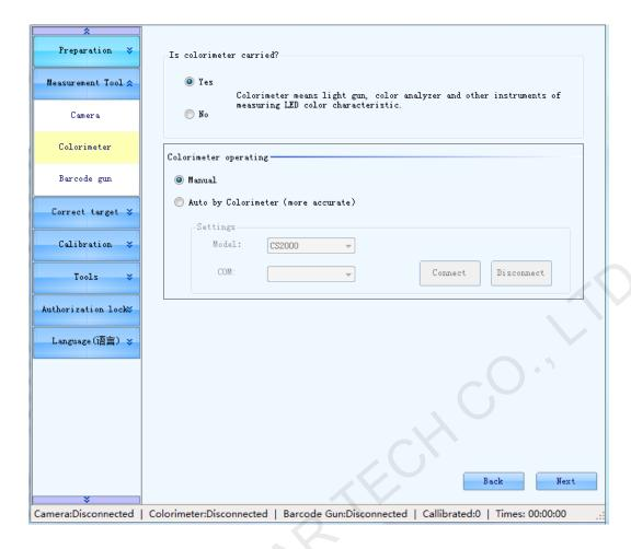
Fig. 4-10 Colorimeter configuration
