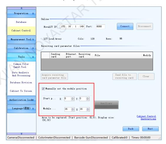
Fig. 5-3 Manually set the location of new module
