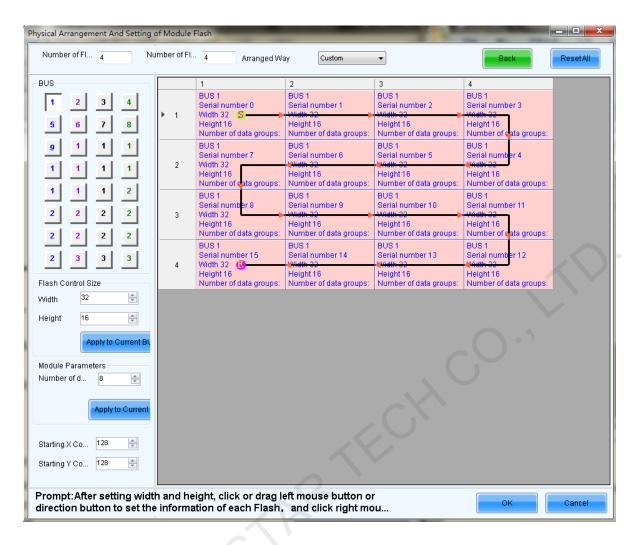
Fig. 4-25 Physical Arrangement and of Module Flash
