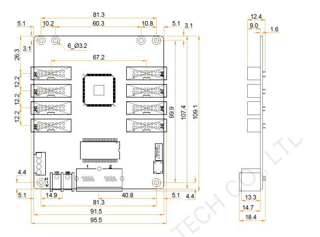
Tolerance: ±0.3 Unit: mm To make molds or trepan mounting holes, please contact NovaStar for a higher-precision structural drawing.
