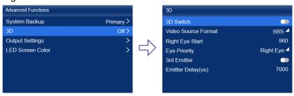
Step 2 Turn on the 3D function by setting the 3D switch to ...
