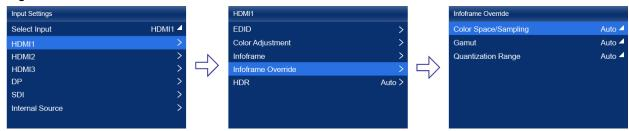
When the device working mode is All-In-One Controller, the **Select Input** menu is not displayed.
