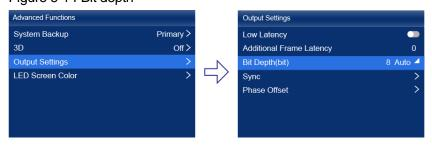
Step 2 Select Bit Depth and then select the desired bit depth value from the drop-down options.
