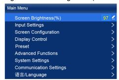
Step 2 Rotate the knob to adjust the brightness to the target value, and then press the knob to confirm.
