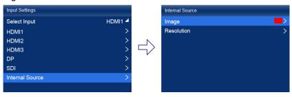
When the device working mode is All-In-One Controller, the Select Input menu is not displayed.
