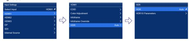
When the device working mode is All-In-One Controller, the **Select Input** menu is not displayed.
