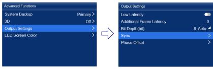
Step 2 Select Sync Source and then select the desired sync source from the drop-down options.
