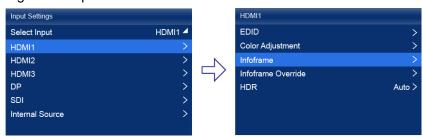
When the device working mode is All-In-One Controller, the Select Input menu is not displayed.
