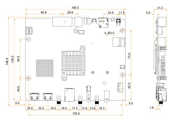
Tolerance: ±0.3 Unit: mm
