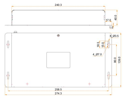
Tolerance: ±0.3 Unit: mm
