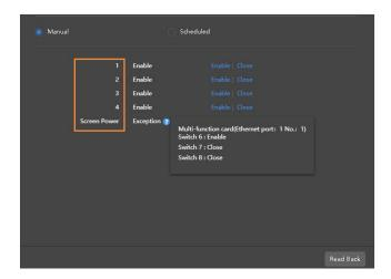
The tags in the orange box can be associated with one or more relay circuits. When multiple relay circuits are associated and each of them is turned on (or off), **Enable** (or **Close**) is displayed. Otherwise, **Mixture** is displayed and the detailed information of each circuit is provided.
