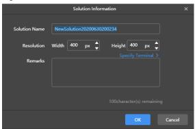
Step 3 Set a name and resolution for the solution, then click **OK** to access the solution editing page, as shown in Figure 3-2.
