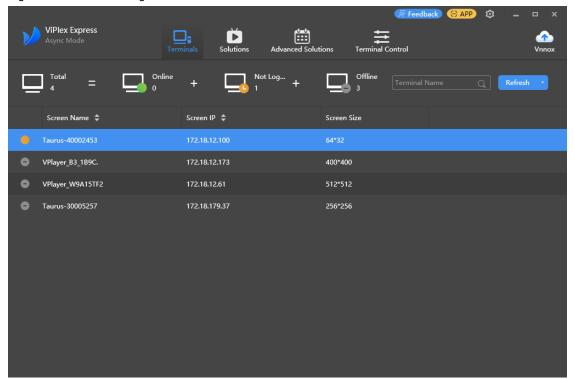
After detecting a terminal, ViPlex Express will try to log in to the terminal with the default account or the account used for the last login.
