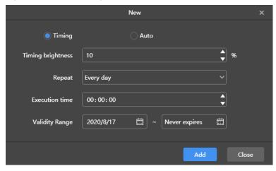
• Automatic brightness adjustment: During the period that you set to enable auto adjustment, the screen brightness will be automatically adjusted according to the automatic brightness mapping table.
